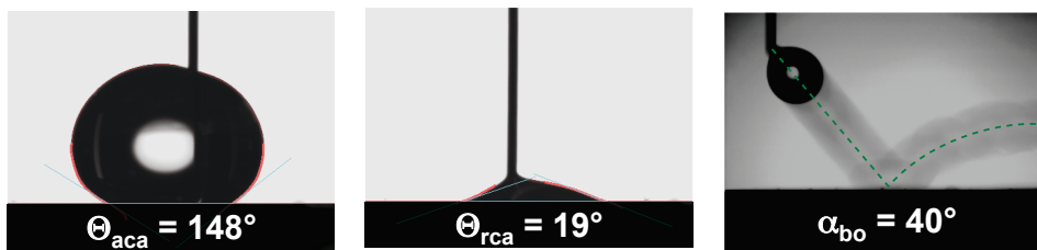
Fig. 7.18: Advancing CA (left), receding CA (center), and bounce-off angle (right) of sample Z10.
