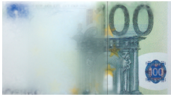
Fig. 7.48: Fogging experiment: Bank note viewed through a glass plate with (half-side) hydrophilic \text{SiO}_2 coating (left, uncoated; right, coated).
