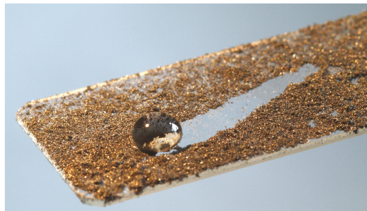
Fig. 7.5: Self-cleaning effect on \text{Al}_2\text{O}_3 sol-gel coating (sample A3) with superhydrophobic properties according to strict theoretical criteria.
