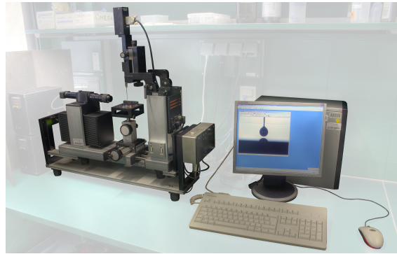
Fig. 3.4: Photograph of the contact angle measurement instrument OCA 20.
