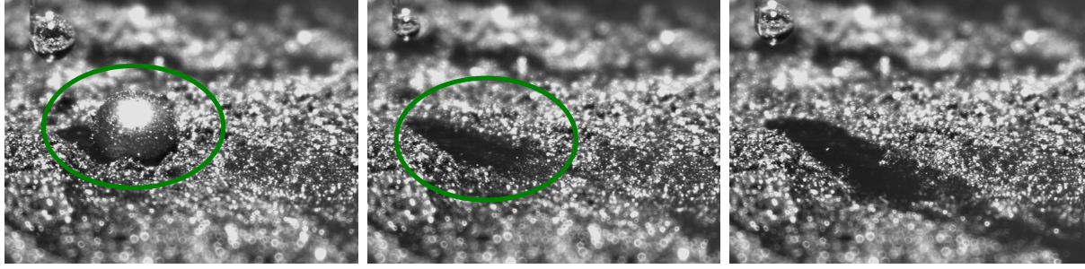
Fig. 7.6: Self-cleaning effect on \text{Al}_2\text{O}_3 sol-gel coating (sample A2) with superhydrophobic properties according to practical criteria. Left: Bounced drop covered with graphite powder. Center: Surface after two bouncing drops. Right: Surface after several bouncing drops.
